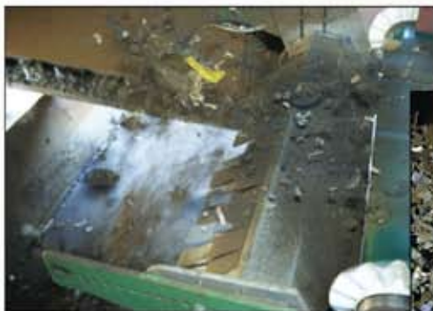
Powerful paddles launch metals into sorting stations
